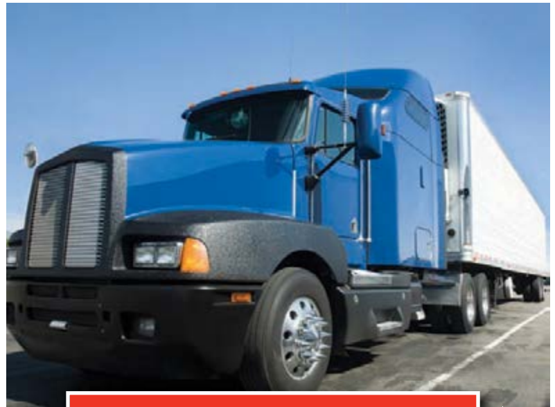
Truck trailers (above) and rail transit cars (below) made of aluminum save fuel costs by reducing weight.
